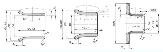
$0.5 \le \beta \le 0.8$   $L1 \le 0.6d \text{ or } \le D/3$  r2 = (D-d))/2  $2t \le D-(d+6mm)$   $3mm \le t2 \le 0.15D$ [A] High  $\beta$  Nozzle  $0.2 \le \beta < 0.5$   $0.6d \le L1 \le 0.75d$   $0.63d \le r2 \le 0.67d$   $3mm \le t \le 12mm$   $3mm \le t2 \le 0.15D$ [B] Low  $\beta$  Nozzle  $0.25 \le \beta < 0.5$   $0.63d \le r2 \le 0.67d$  t = 0.25d t = 38mm[C] Low  $\beta$  Nozzle, with Throat Tap
